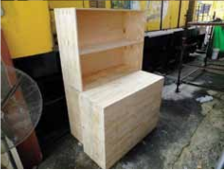
Under the direction of our carriage builder, Brian Edwards, cupboard skins have been fabricated and are being moved into BE 346 for installation
