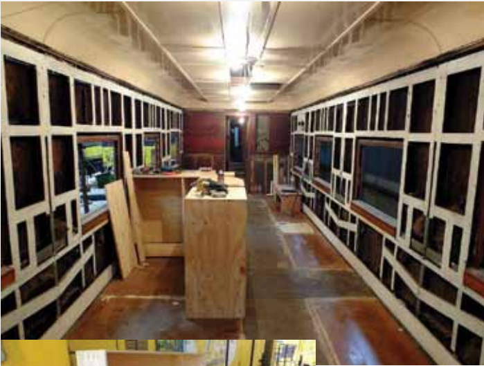
Under the direction of our carriage builder, Brian Edwards, cupboard skins have been fabricated and are being moved into BE 346 for installation
