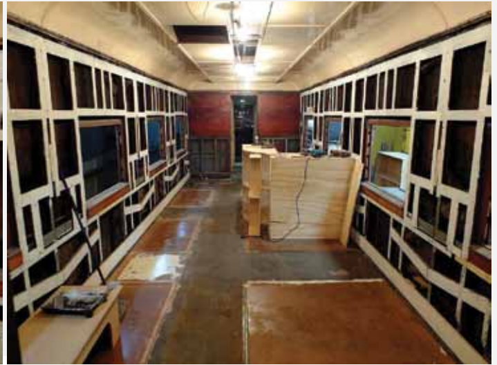
Under the direction of our carriage builder, Brian Edwards, cupboard skins have been fabricated and are being moved into BE 346 for installation
